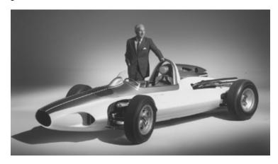
Duntov is shown here, proudly posing with his 1959 CERV (Chevrolet Engineering Research Vehicle) I, clearly a racing-oriented concept intended to test advanced designs and components for future use. The CERV's independent rear suspension was adapted to the 1963 Corvette. It's 350 hp 283 CI V8 featured aluminum block and heads, and fuel injection. A grand start to a long series of exciting Corvettes, even if they never made it into production.
