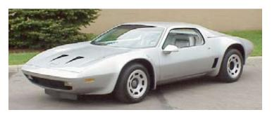
The early seventies were heady times for the experimental Corvette development group, with concepts flying out left and right. The XP-895 was an experiment in using aluminum extensively, although heavily based on the 2-Rotor. But it used a conventional (presumably aluminum) 400 cid V8, and weighed some 400 lbs less than its steel donor. But plain old cast-iron and fiberglass production Corvettes were flying out the dealers' doors, so there was little incentive to rock the boat.
