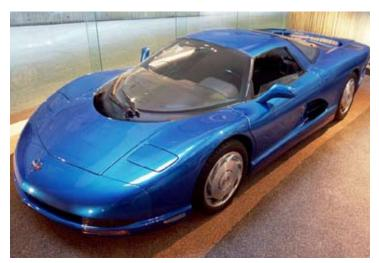
The Indy concept was developed into the CERV III of 1990, designed to be (another) world-class top-level sports car, but this one was taken towards being more production ready (or am I just stirring up old rumors?). It's 650 hp twin-turbo LT-5 engine left little doubt as to its capabilities. The car was built by Lotus, using carbon fiber extensively. Final cost estimates to produce it: \$400k. Never mind; once again.
