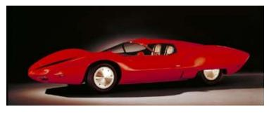
It's a little sketchy as to what exactly defines a Corvette concept or not. The CERVs weren't actually called Corvettes, nor was this ultra-low Astro 1 from 1968. But all the mid-engined concepts were in some related to the Corvette idea, this one exploring the outer limits of aerodynamic drag reduction for a sports car, as well as alternative power plants. The Astro 1 featured a modified Corvair flat six, making 240 hp.
