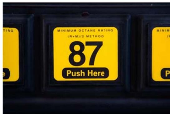
The compression ratio of your engine determines the octane rating of the gas you must use in the car. One way to increase horsepower of an engine of a given displacement is to increase its compression ratio. So a “high-performance engine” has a higher compression ratio and requires higher octane fuel. The advantage of a high compression ratio is that it gives your engine a higher horsepower rating for a given engine weight. It costs more to run, though.
