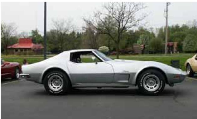
A body-colored rubberized front bumper took up residence on the 1973 Corvette, replacing the chrome strip used previously. Furthermore, the side vents were now single, almost vertical, openings and radial tires were standard for the first time. And power dropped again, with the base 350 now rated at 190 horsepower and a new optional "L-82" 350 made 250 horsepower. The sole 454 was an "LS4" rated at 275 horsepower.
