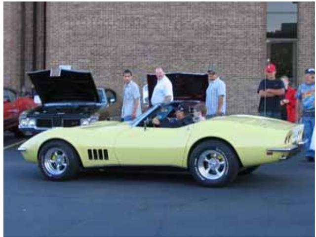
Again there were coupe and convertible Corvettes offered for 1968. The convertible again stowed its top under a hinged hard cover while the coupe featured swooping buttresses on either side of a tunneled-in rear window. The most unique element of the coupe, though, were the two removable roof panels -- the first "T-tops."
