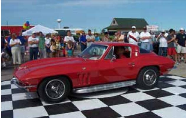
Visually, the easiest way to tell a 1965 Corvette from a '64 is the three functional vertical louvers in each front fender. But the big news (literally) was the availability of the new 396-cubic-inch big-block V8. And there was even better news as four-wheel disc brakes became standard (though 316 fools did delete them in favor of drums and a \$64.50 credit).
