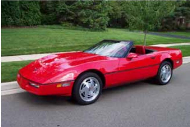
New 17-inch wheels inside P275/40ZR17 tires were added to the 1988 Corvette options list while new aluminum cylinder heads and a revised camshaft boosted the L98 to 245 horsepower with even better torque characteristics. This was also the last year Chevy would foist the dreadful 4+3 transmission off as the shift-it-yourself choice. A 35th anniversary model, done in a white-on-white scheme, marked this milestone.
