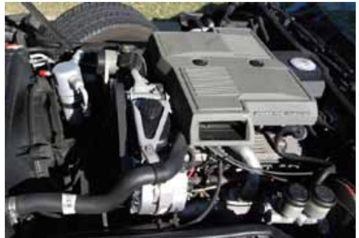
air to the underhood ducts, making the ‘84 a “bottom-breather” like the Shark before it. The engine compartment was color-coordinated in silver and black. Palmer even persuaded GM’s AC-Delco Division to develop an appropriately styled battery.
