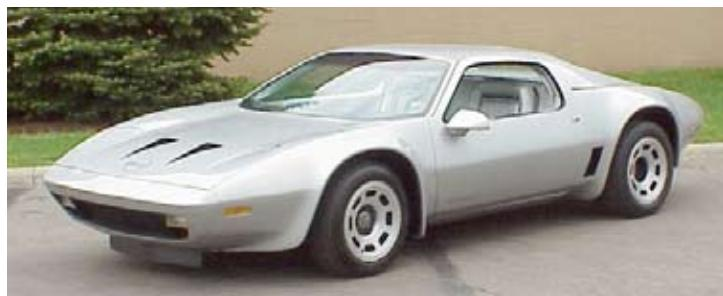
The early seventies were heady times for the experimental Corvette development group, with concepts flying out left and right. The XP-895 was an experiment in using aluminum extensively, although heavily based on the 2-Rotor. But it used a conventional (presumably aluminum) 400 cid V8, and weighed some 400 lbs less than its steel donor. But plain old cast-iron and fiberglass production Corvettes were flying out the dealers' doors, so there was little incentive to rock the boat.
