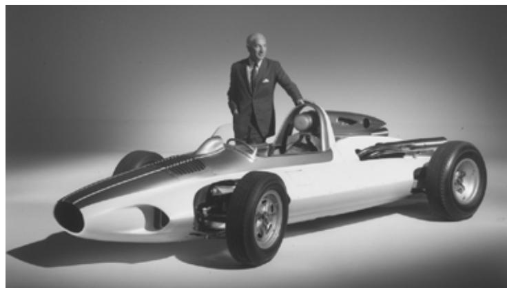
Duntov is shown here, proudly posing with his 1959 CERV (Chevrolet Engineering Research Vehicle) I, clearly a racing-oriented concept intended to test advanced designs and components for future use. The CERV's independent rear suspension was adapted to the 1963 Corvette. It's 350 hp 283 CI V8 featured aluminum block and heads, and fuel injection. A grand start to a long series of exciting Corvettes, even if they never made it into production.
