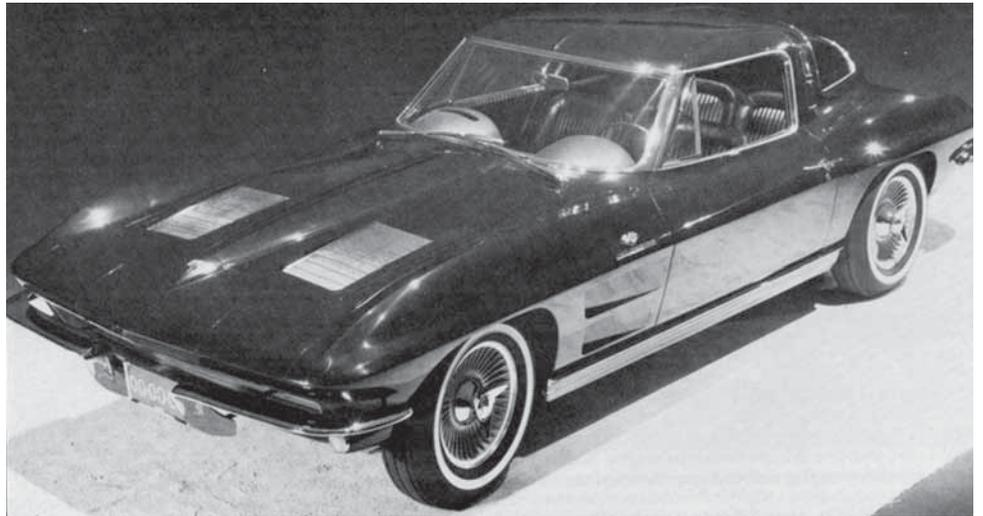
Designer Larry Shinoda was given project and stretched the already penned 2-seat midyear coupe to accommodate the back seats and the extra legroom required. Six inches was added to the C2's wheelbase to stretch it out to 104 inches. The pictures below show that the four-seater Corvette's doors are much longer and shaped differently than the production 2-seater. The roof is also slightly taller and the rear glass looks to be longer as well.
